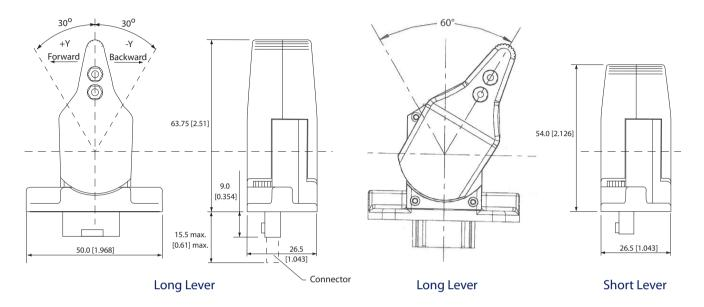
Joystick fitted with 2 x M3 inserts Maximum screw penetration 6 [0.236]
